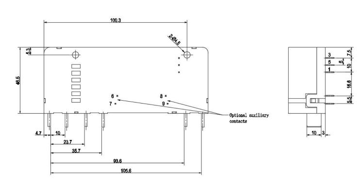
Remark:(1)In case of no tolerance shown in outline dimension:outline dimension≤1mm,tolerance should be±0.2mm;outline dimension>1mm and <5mm,tolerance should be ±0.3mm;outline dimension≥5mm,tolerance should be ±0.5mm.
